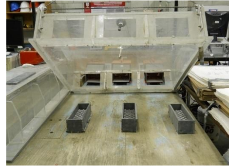
Figure 1: Plastic shrinkage test set up
